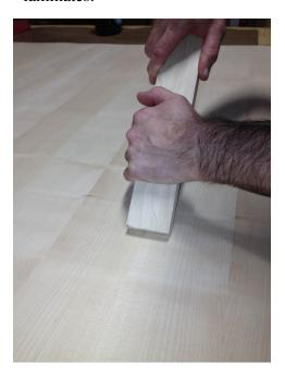
3. Use the stiff scraper for maximum contact pressure. J-rollers and hammer blocks do not allow you to make the most of your body weight when you make contact by hand power.
